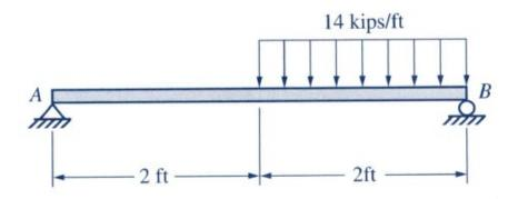
13-22 to 13-37 Refer to Figs. P13-22 to P13-37. Construct the shear force and the bending moment diagrams for the beam in each figure due to the loading shown by using the relationships among the load, shear, and moment diagrams.
